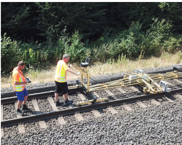
Measuring the track geometry using the EMA uni
