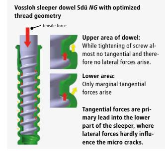
Torque tests simulate the tightening of the screw in the track; first results show: the use of Vossloh dowels Sdue NG in sleepers without dowel reinforcement leads to a reduction of crack growth of more than 60 %.
